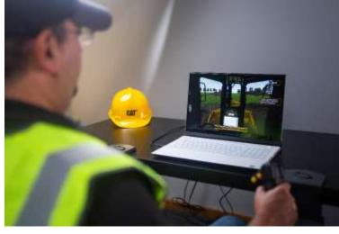
every time an exercise is undertaken. For example, when backfilling a trench with a Dozer, the operator must fully load the blade with material; push material to the trench with the Dozer in the perpendicular position; complete with a minimum number of passes; and allow extra material for compaction, staying within 6" of the existing grade. The student must think each step through while using the simulator for a successful session. Decision-making must be concrete during simulation sessions.
